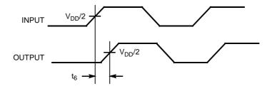
Figure 7. Device-Device Skew
